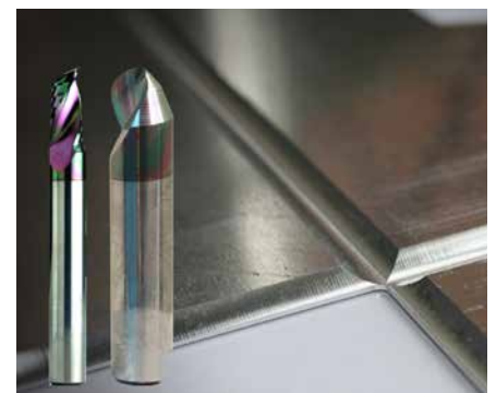
3mm aluminium routed and grooved with MP Superior tools
