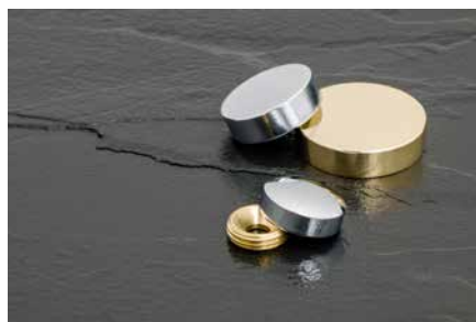
The brass collar is surface mounted with a 4mm countersunk screw with the decorative cap applied to the collar.
