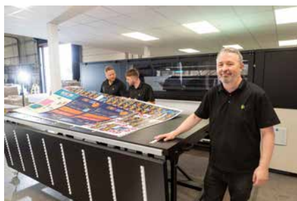
The Hybrid Jeti Tauro H2500 LED relies on UV LED curing to offer six vivid colours plus white print
