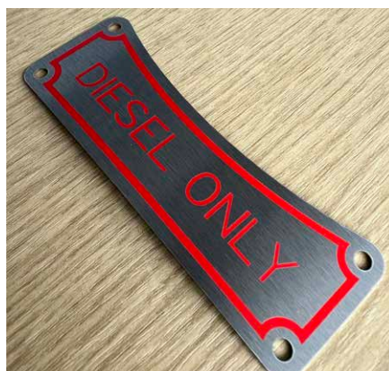
Chemical etched with painted infill is then lacquered and stoved to a high temperature
