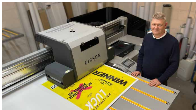
The Gibson 3200 hybrid roll/flatbed printer uses the latest 6th generation Ricoh print heads
