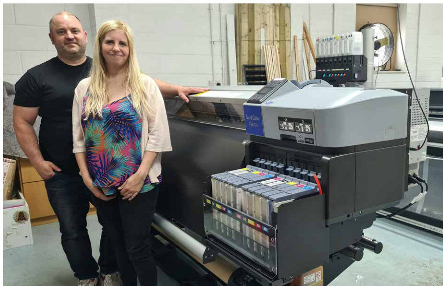
The Epson SureColor SC-F9400H is a fast, high volume, six-colour, 64 inch paper transfer sublimation printer, suitable for sports and fashion
