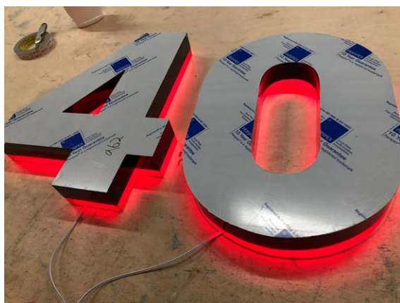
Built up acrylic Letters, two tone returns (Black and Clear) with Red side and Halo Illumination
