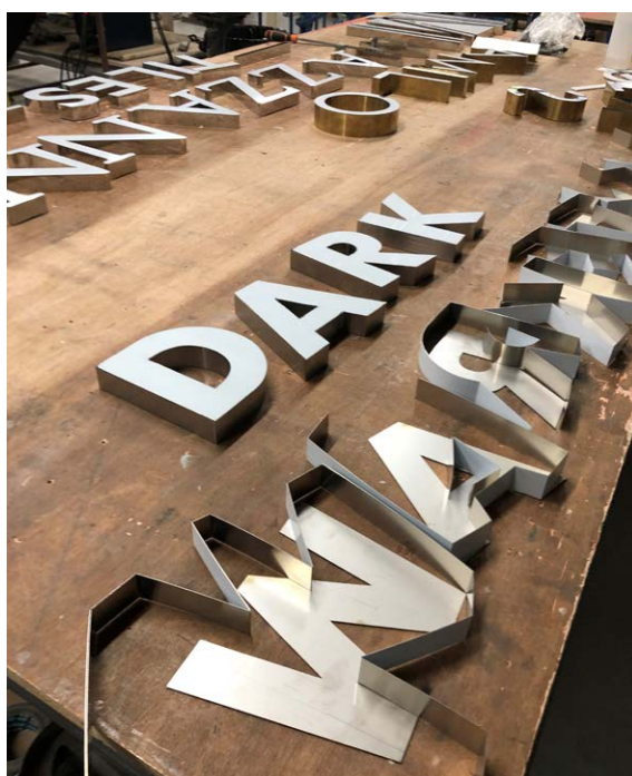
1.2mm Stainless Steel faces with 0.8mm Stainless Steel returns
