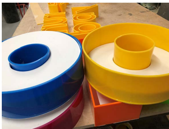
3mm Acrylic Faces with 3mm returns, 10mm foam backs
