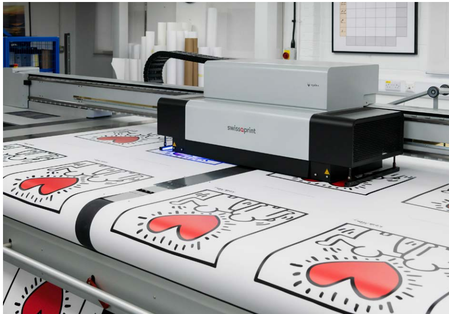
The 3.2 m flatbed Nyala 4 with roll to roll and dual roll functions has enhanced performance and productivity in one acquisition.
