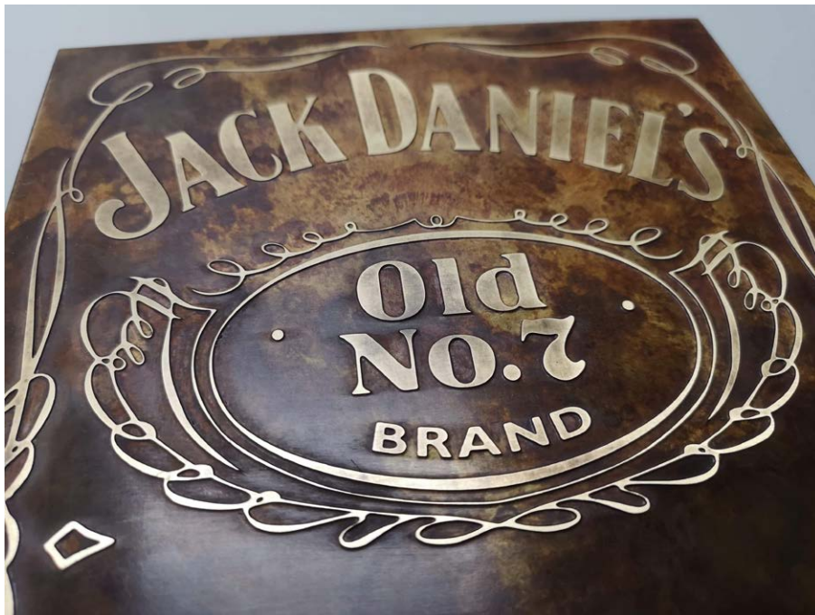
Chemical reverse etching and patination creates a range of amazing looking finishes
