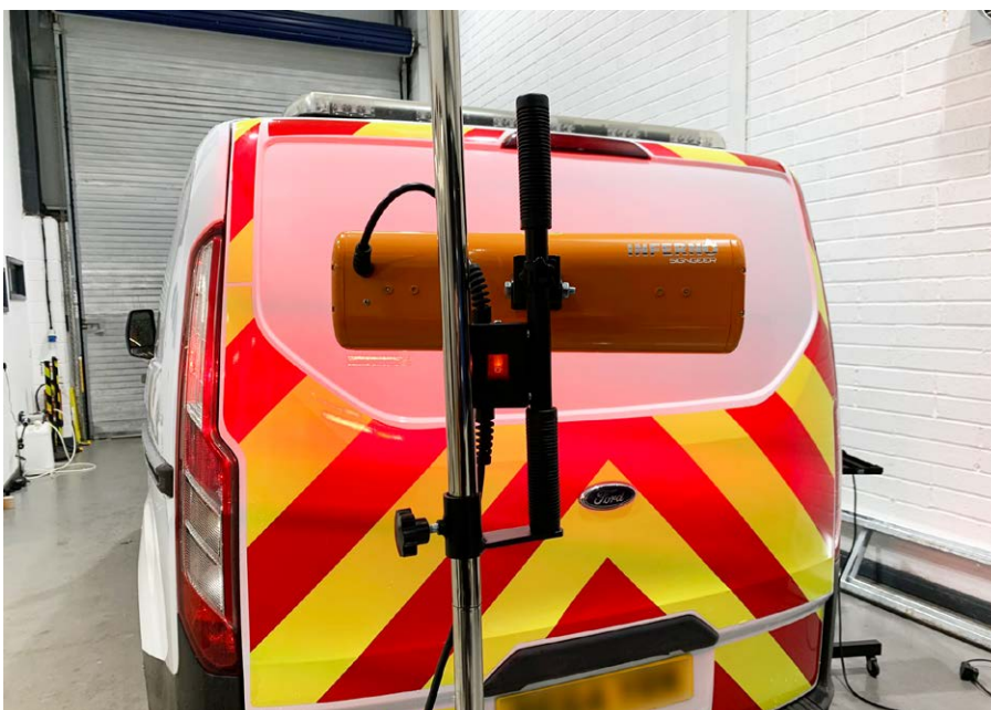
The Inferno Infrared Heater from Signgeer is a great aid for generalised preheating of panels prior to sign-writing or removal
