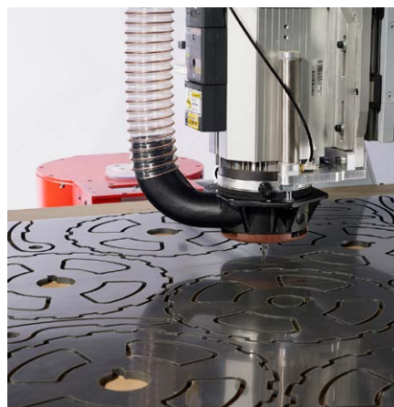
XYZ 4020 incorporates the latest helical rack and pinion drive system
