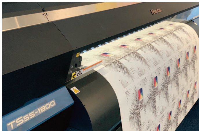
The dye sublimation process - material is printed on a Mimaki and is then heat pressed onto the fabric.
