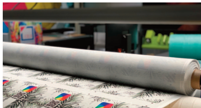
The dye sublimation process - material is printed on a Mimaki and is then heat pressed onto the fabric.
