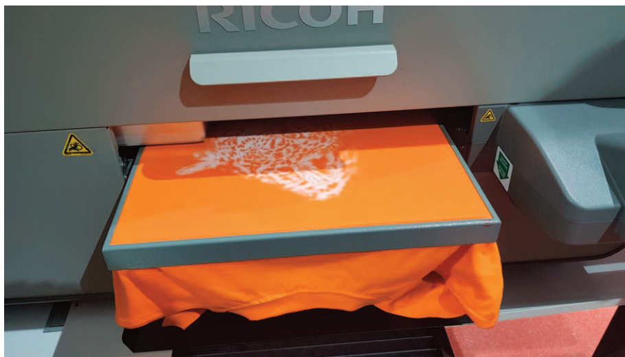
Ricoh's eco-friendly inks include white, perfect for printing a base layer on dark fabrics
