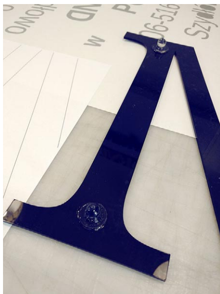
Using the correct adhesive for acrylic/foam or two-part methacrylate for ACM apply the selected size of locator to each letter.
