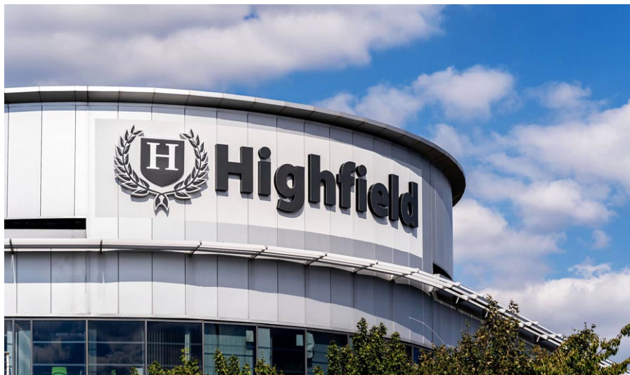
The sign for the exterior of the building, which is black by day and changes colour by night includes a logo made from aluminium, acrylic and internal RGB LED illumination.
