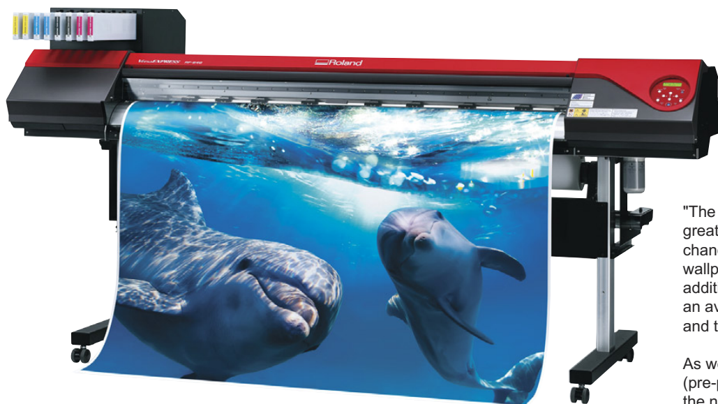
Wallpaper Ink runs its two Roland VersaEXPRESS RF-640 inkjet printers and Roland cutting systems 24 hours a day to produce made-to-measure wall graphics
