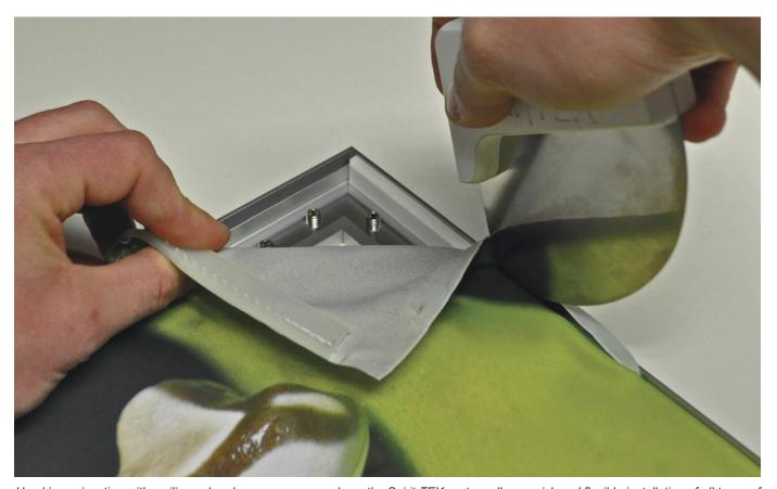
Used in conjunction with a silicone bead on one or more edges, the Spirit-TEX system allows quick and flexible installation of all types of soft signage fabrics
