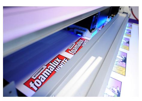
A variety of substrates used within the digital print industry including foam PVC sheets can be especially sensitive to the effects of static
