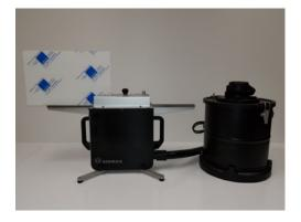
table-top machine is suitablel for the edgepolishing of a wide range of acrylic and PMMA substrates, enabling a superior quality high gloss or matt finish using either a synthetic or natural diamond polishing tool. Weighing 15kg and with outer machine dimensions of 420 x 360 x 390mm, the BOX will handle materials up to 20mm thick at a feed rate of up to 1.5 metres/minute and at variable milling motor speeds from 7,000 up to 12,000rpm to accommodate different materials.
