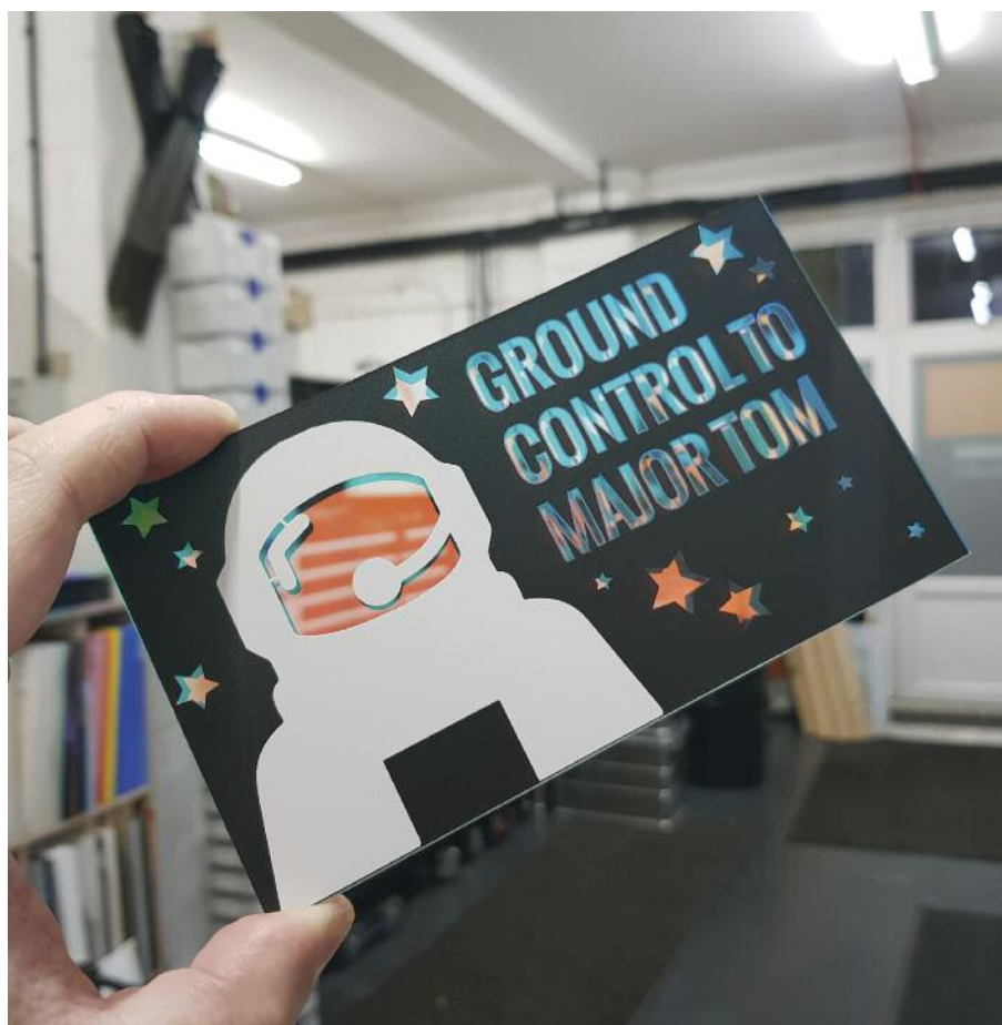
Printing a bottom layer of white ink makes colours on top really pop, while the gloss ink option enables spot gloss or matt finishes and touchable embossed effects
