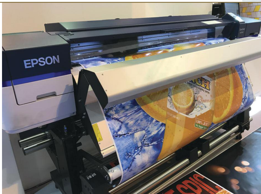
The SureColor SC-S60600 operates with four to 10 colours and offers up to 95.3m 2 /hr single-pass productivity.
