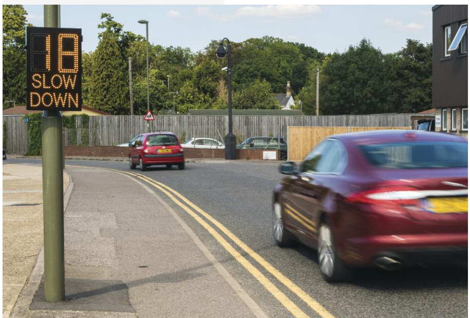
An effective way to calm traffic – Speed Awareness Message (SAM) signs display the driver's exact speed in real time
