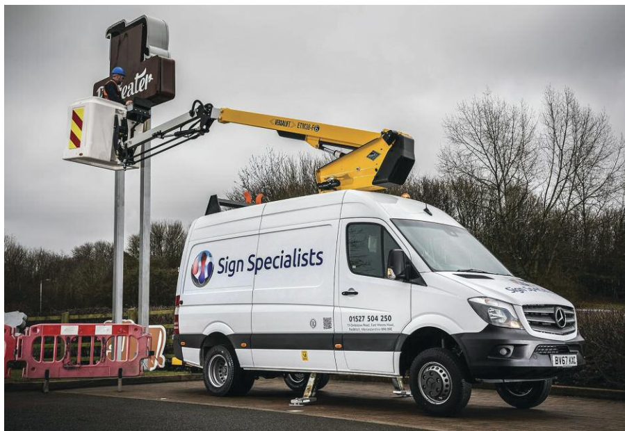
Sign Specialists' new Sprinter 514 CDI is fitted with a 'cherry picker' that allows operatives to work safely at heights of up to 14.3 metres
