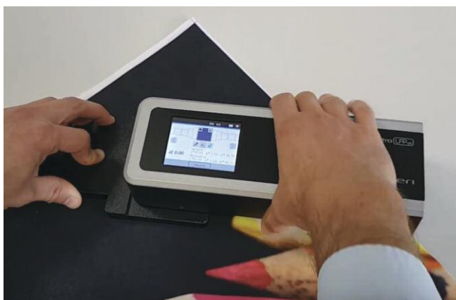
The detachable spectral unit delivers reliable spot measurements
