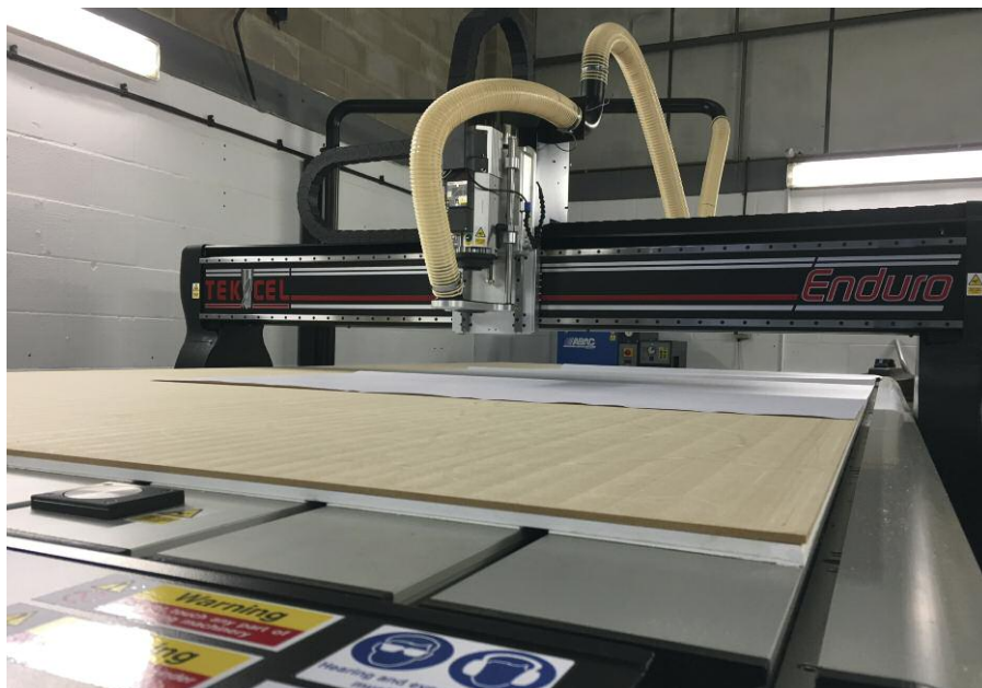
Installation of a Tekcel 4m x 2m flatbed CNC router is part one of a four-phase plan for updating and improving the production centre
