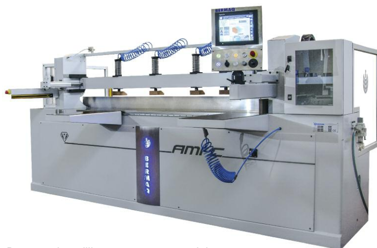
The Bermaq: the milling motor moves and the acrylic stays still, just as it does on the Homag machine, pictured page 59 middle left
