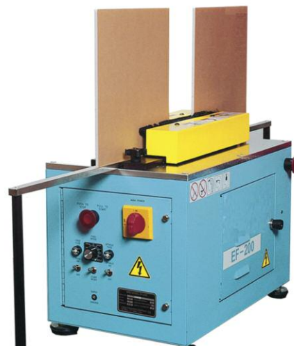
The EF-200 diamond polisher: acrylic moves across the milling motor
