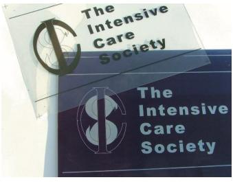
To etch a sign you must first use a film to create a stencil on the metal surface
