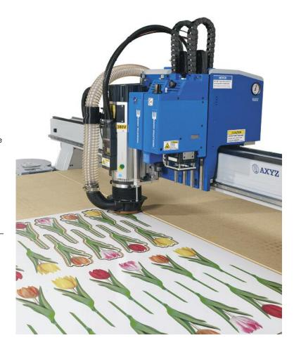
of frequently problematical thin materials such as vinyl, cardboard and paper and thicker and heavier materials such as aluminium and other non-ferrous metals, ACM (Aluminium Composite Material), acrylic and foamed boards.
