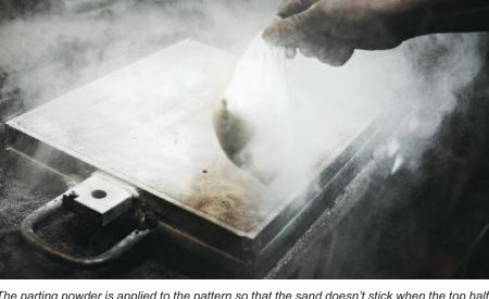
The parting powder is applied to the pattern so that the sand doesn't stick when the top half of the mold is produced in sand
