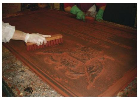
A sand-cast sign that has cured and been taken out of the sand box: the surface sand is being removed before the whole sign is sand blasted clean.
