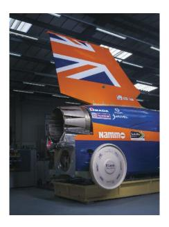
The BLOODHOUND SSC is designed to not only go faster than the speed of sound but up to speeds of 1,000mph, covering a mile in just 3.6 seconds. The tail fin provides a vital part of the supersonic car, providing stability that can withstand the use of both a jet and a rocket to produce more than 135,00bhp.
