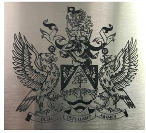
Chemical etching can reproduce fine detail that would be very expensive to engrave
