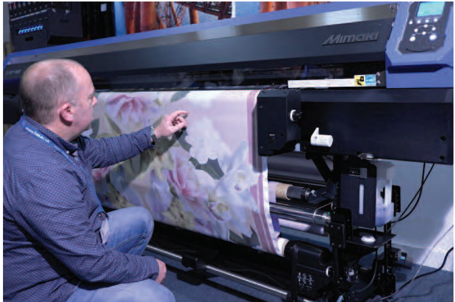
Dr Roger Spark examines printed cloth on the new Mimaki Tx300P-1800 digital textile printer.
