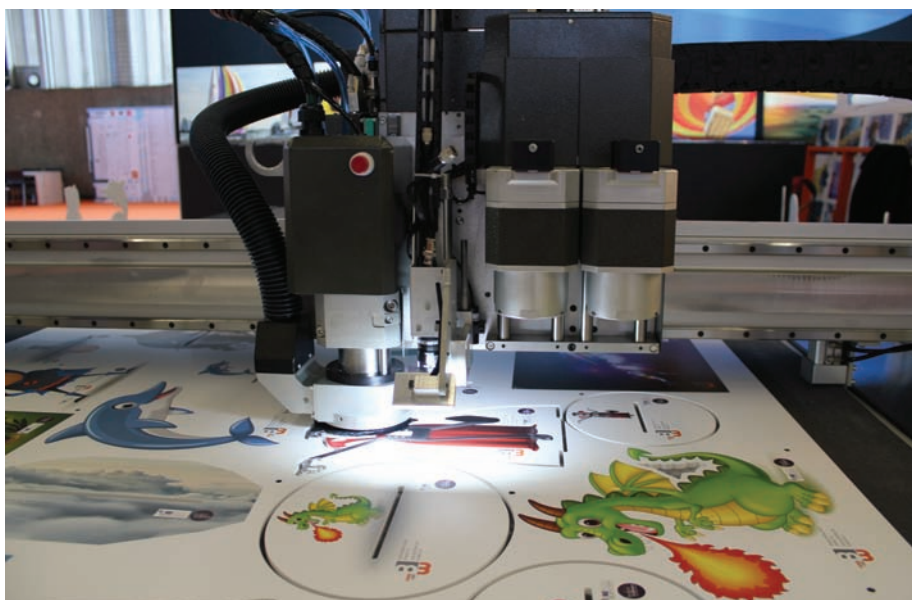
The Versa-Tech offers a 1.6m cut width with router and laser tooling options.
