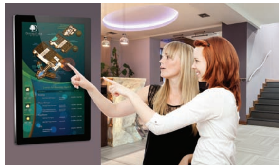
PCAP screens have the sensor behind the glass.
