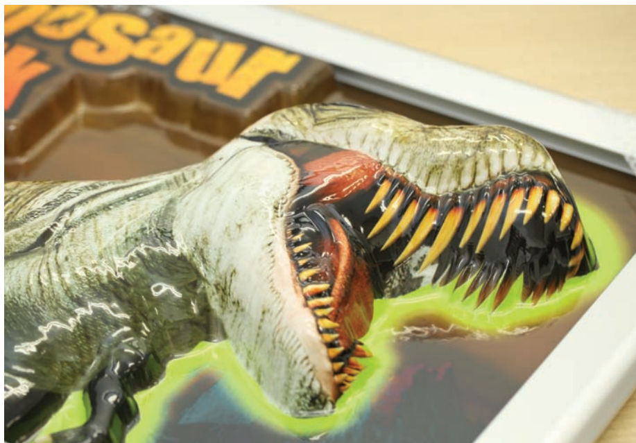
This new ink technology allows thermoformed objects to be imaged before forming.
