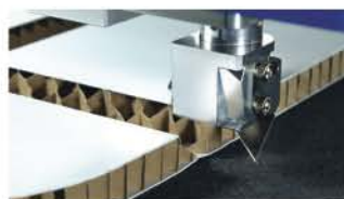
XVT - V cutting tool, perfect for POS and displays using honeycomb board.
