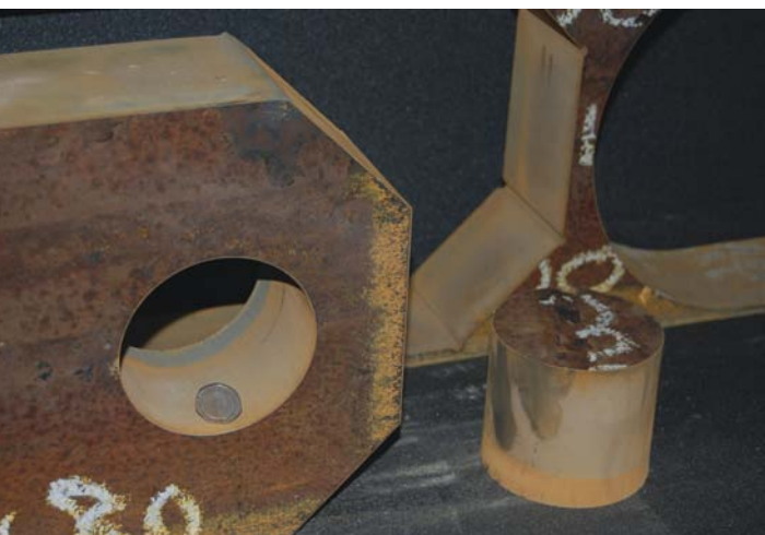
A 20p piece demonstrates the sheer depth that can be cut using the water.
