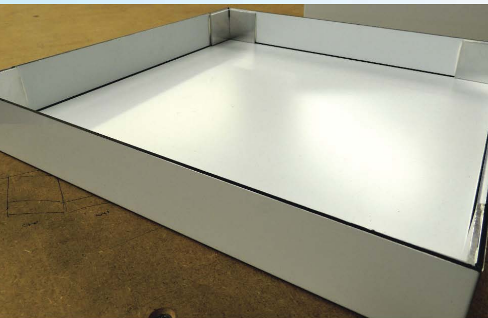
NE Plastics make trays from their own brand of Aluminium Composite, Alliance.
