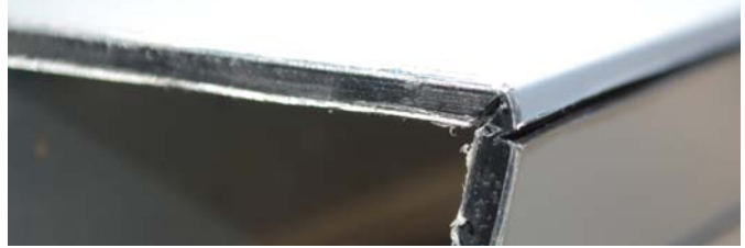
V-grooved, folded with just the excess left to be removed.
