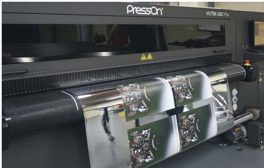
PressOn's EFI VUTEk QS2-Pro is particularly competent when working with traditionally tricky materials that benefit from the highly opaque white coverage.
