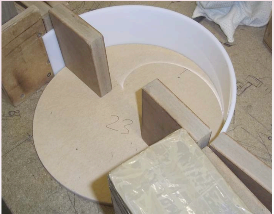
The acrylic is bent to form the letters.
