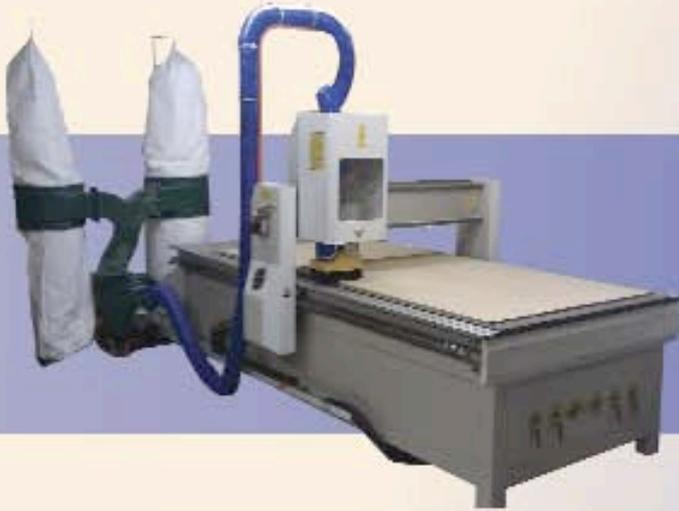
Model M25 (1300 x 2500 x 200mm) including 4.5 KW water cooled spindle, vacuum table, dust extraction, Vcarve software, DSP Handle etc... delivery on site, set-up/training £ 11,415.00 +VAT
