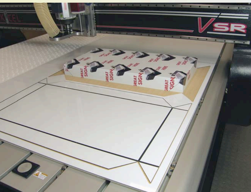
Many trade suppliers use Tekcel routers to produce sign trays in volume.
