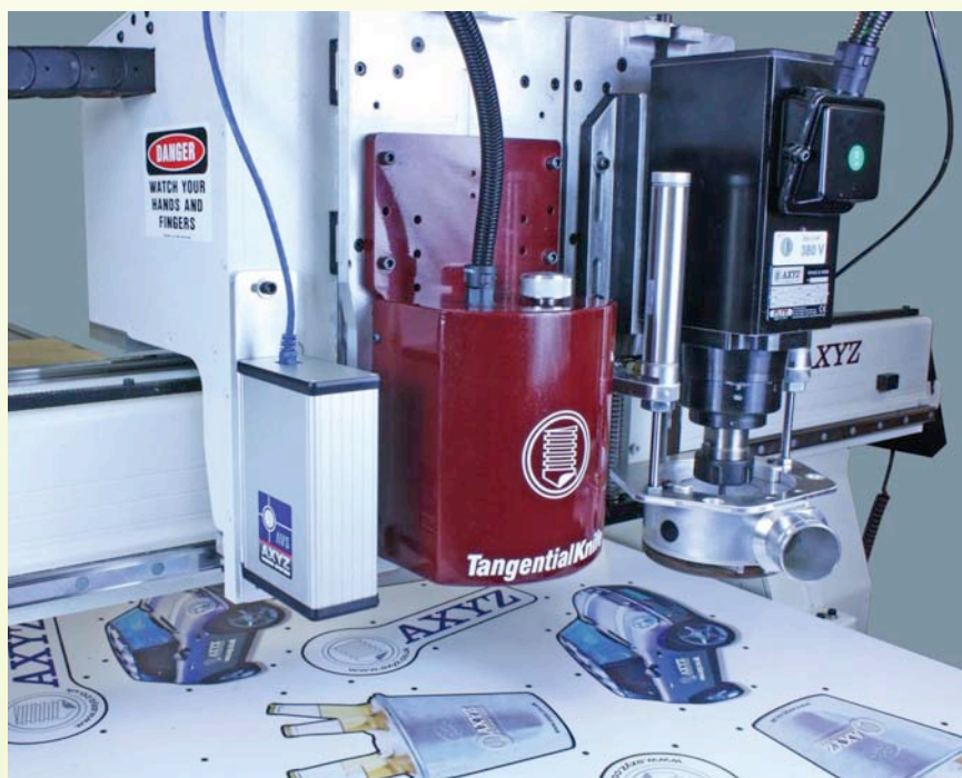
Precision alignment for cutting out pre-printed materials with XYZ's AVS camera registration system.
