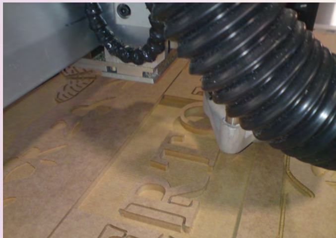
Your Sign Company's in-house Gerber Sabre router begins to create the 3D sign.
