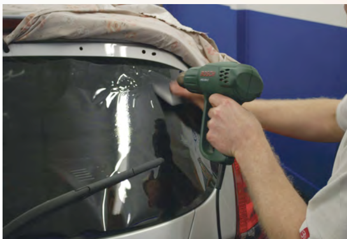
Tom heats the film until it starts to physically change and he can shape it to the outside of the window.
