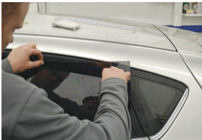
This new model Fiesta is a first for Tom so he's cutting the window film to shape and size as he goes along.
