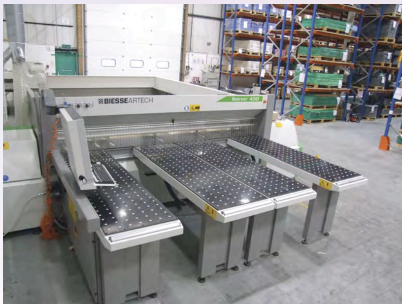
The beam saw can accommodate sheets 3m x 2m in size.
