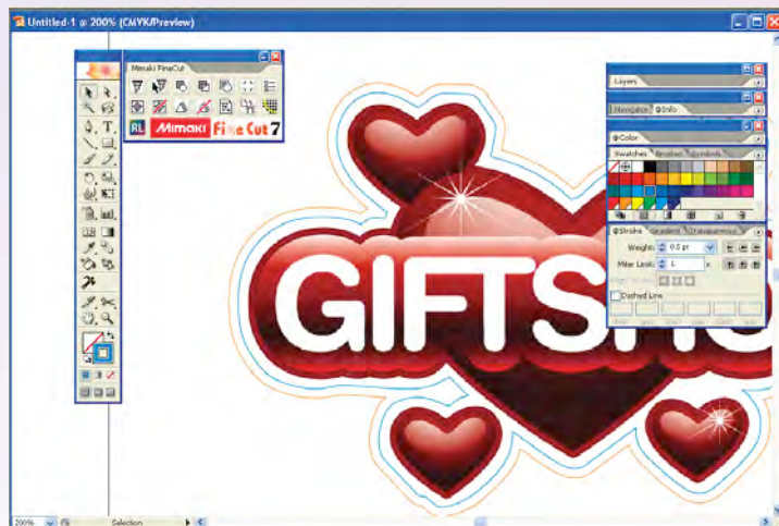
A screenshot from Mimaki's free cutting software (FineCut) showing the image to be printed and half cut.
