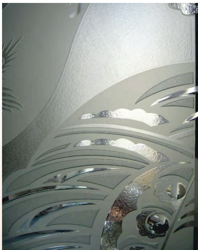
An example of French Embossing, the corroding of glass with an acid to produce a great variety of tones, textures and decorations.
