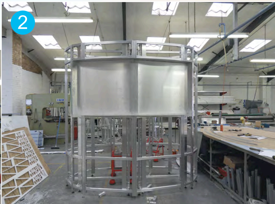
Step 2 showing the internal frame as the sections are put together.
