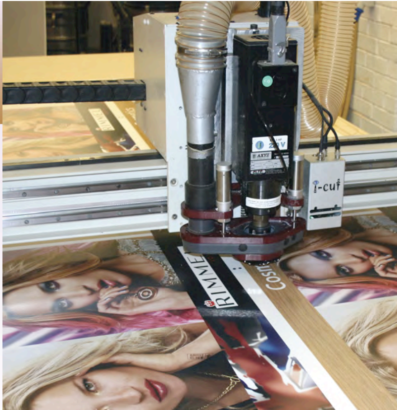
This close-up shows the print-and-cut capabilities now possible with XYZ routers.
