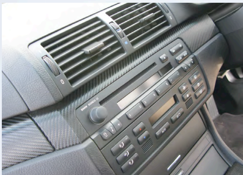
The Metamark MM-CF4 film is very heavily textured and constructed from multiple layers of cast film.
