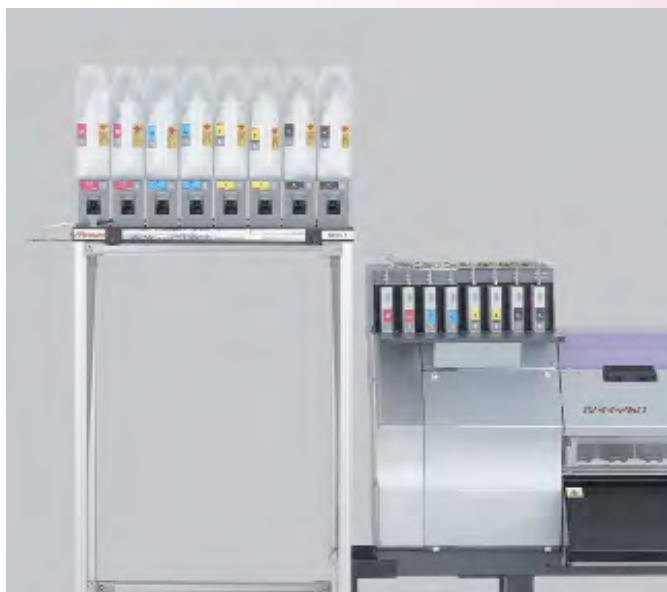
The two litre ink sacks tackle the environmental issues that are commonly linked to plastic cartridges.
