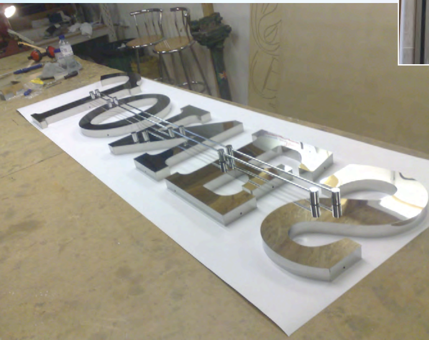
Built up s/steel letters with fitted Gdi Trax rod connections.
