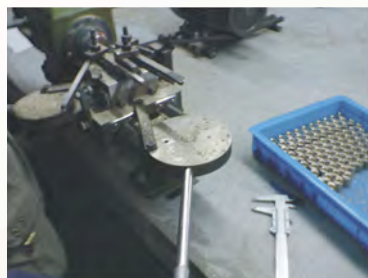
Cut lengths are drilled and threaded.
