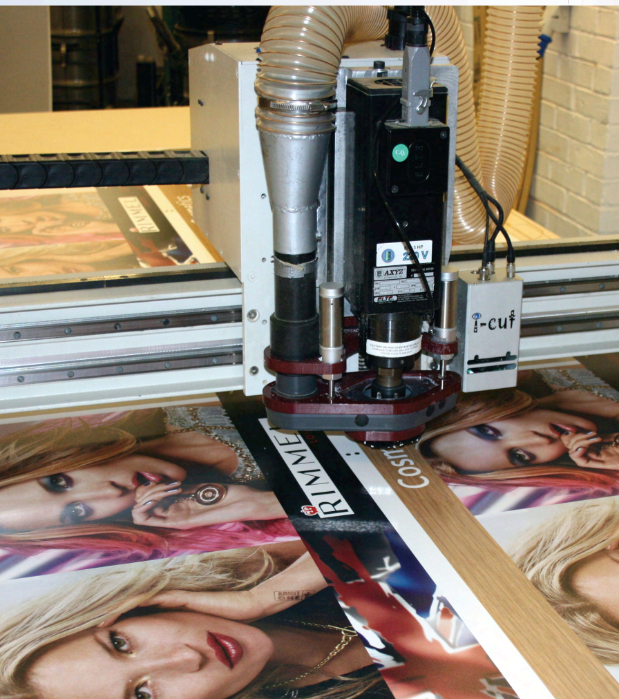
The Intelligent Cutting System (ICS) can now be attached to any standard AXYZ International router to cut digitally-printable media.
