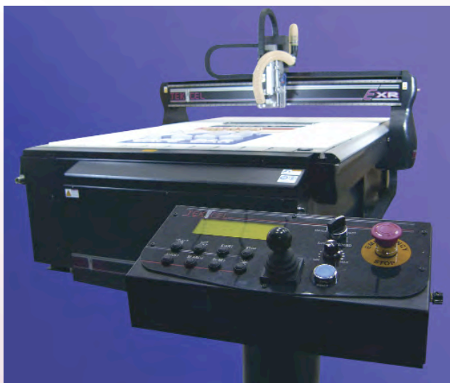
Tekcel's new control post now has a user friendly joystick control podium mounted as standard.
