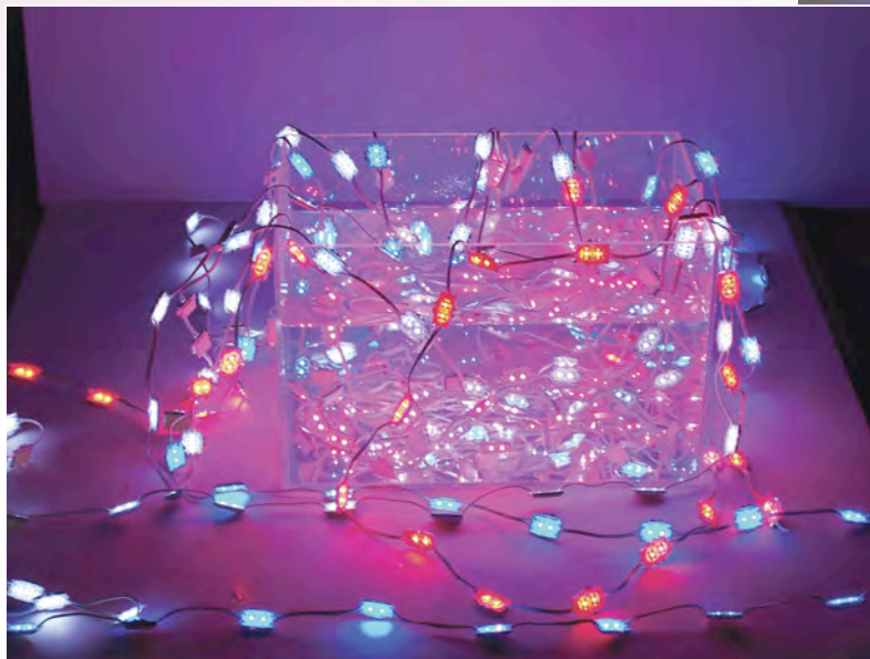
S.M.P.'s waterproof LEDs in action. Rated to IP68 these can be immersed in water up to a pressure depth of one metre.
