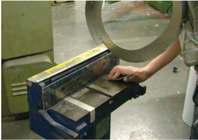
End of return being trimmed to length before soldering.
