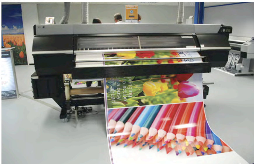
The Seiko II ColorPainter offers true 720x720dpi resolution at impressive speed.
