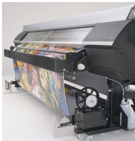
The roll take-up unit with four winding modes comes as standard. Left to right: Tension/Outer Take-up, Tension/Inner Take-up, Loose/Outer Take-up, Loose/Inner Take-up.
