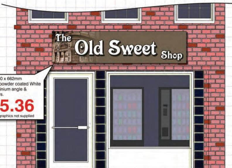
Aluminium Tray 2950 x 662mm with 50mm returns powder coated White complete with aluminium angle & colour coded screws.
